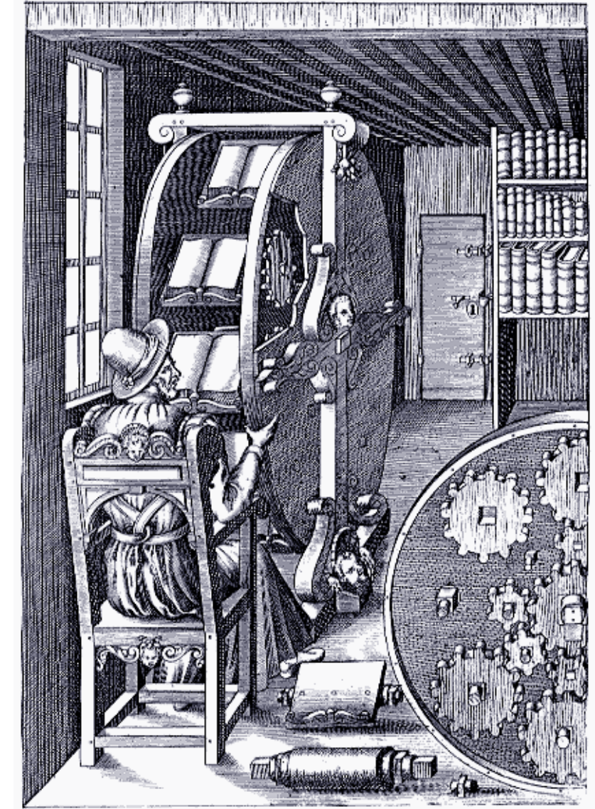
The bookwheel was designed to allow a user to read and compare multiple books, without having to repeatedly open and close the books.
